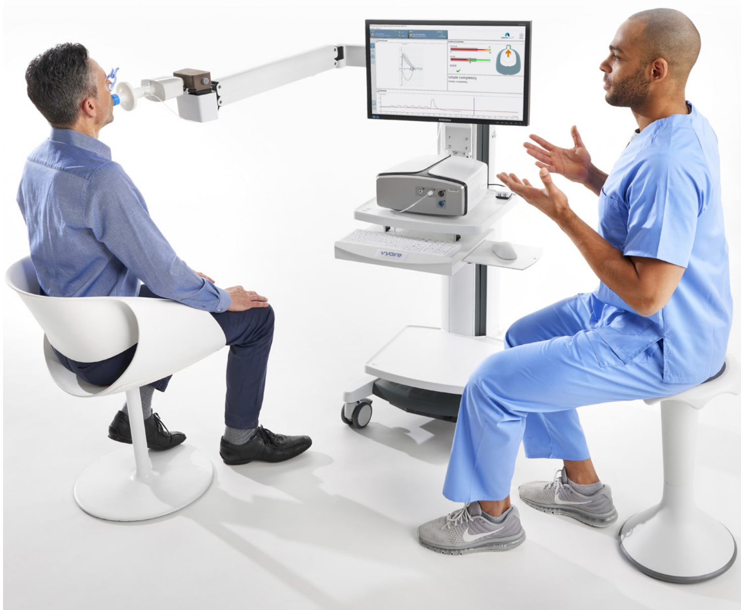
Vyntus ONE with ultrasonic flow sensor technology to perform slow and forced spirometry, SB diffusion, N 2 -washout lung volumes, CPET and many more.
