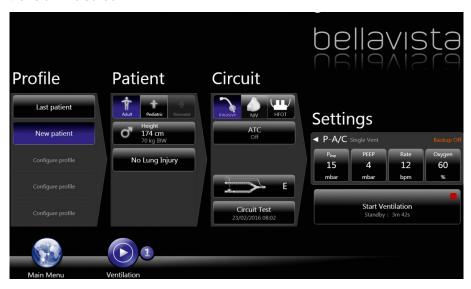
Every time you have changed a flow sensor or a breathing circuit, perform a flow sensor and leak test. To ensure that the test is performed properly it is essential that you select the breathing circuit used on the start screen.
