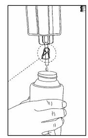
Figure 2–13: Draining water trap
