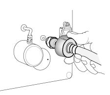
Figure 2–29: Connecting the O2 Hose
