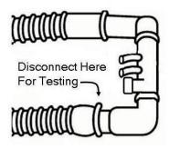
Do not disconnect the Nasal CPAP device at the wye and leave the prongs open to ambient.
