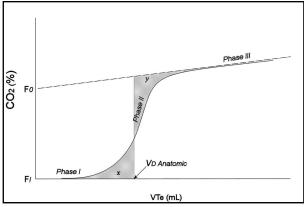
Using Fowler's nomenclature, phase I is the initial exhaled volume with constant  $FCO_2$ .  $FCO_2$  during phase I is calculated as FI. Phase III is the linear part of the capnogram associated with exhalation of gas from the lung gas exchange units. This is calculated using linear regression over that part of the capnogram representing 30 to 70% of exhaled  $CO_2$ . The slope of phase III is calculated as m, with offset at the  $FCO_2$  axis FO.
