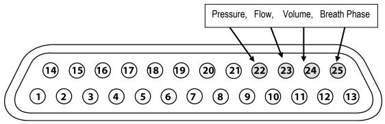
Figure 2–37: Analog Outputs Pin configuration
