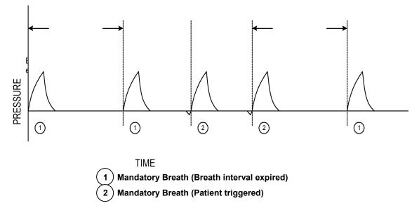
Figure 3–13: Assist Control Ventilation Waveform
