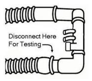
Figure 6–3: Disconnect Point for Calibration
