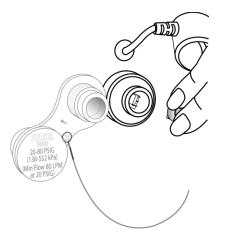
The oxygen sensor cell is located on the rear panel, between the two gas fittings. The oxygen sensor cable emerges from the rear panel directly above the sensor. Carefully align and then gently push the connector onto the oxygen sensor until it seats. When a good connection has been made, slide the protective cover down and push over the sensor.
