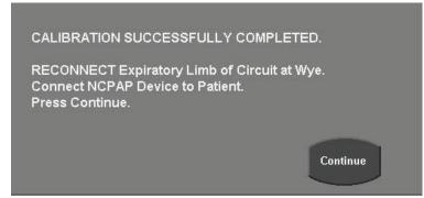
Figure 6–5: Calibration Successfully Completed Screen
