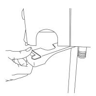
Rotate the metal locking lever on the lower right of the ventilator body forward to an open position.
