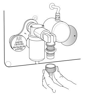
Attach the Air supply hose to the "Smart" connector fitting with the integral water trap/filter on the left of the back panel as shown in Figure 2–31.
