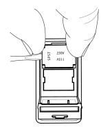
4. The fuse holder contains two fuses, 3.1 amps (for 100/120 volt lines) and 2.0 amps (for 230/240 volt lines) as shown in Table 8–1.
