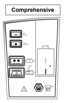
Figure 2–19: Avea Front Panel Configurations Standard and Comprehensive
