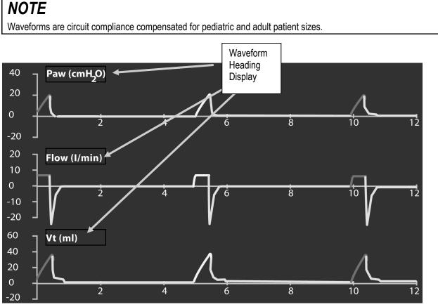
Figure 4–1: Waveform Graphs Displayed on the Main Screen
