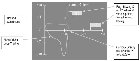
Figure 3–2: Flow/Volume Loop in Freeze Mode
