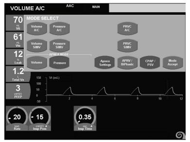
Figure 3–21: Pressure Apnea Backup settings for CPAP Mode
