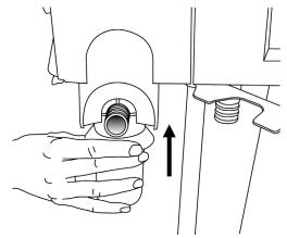
Figure 2–7: Insert exhalation filter
