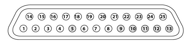
Figure 2–34: Analog Ground Pins
