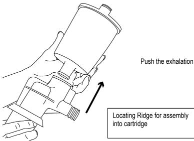
Push the exhalation filter into the water trap assembly top as shown.
