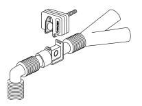
Figure 5.5b Pediatric / Neonatal Adapter Figure 5–5: Airway adaptors
