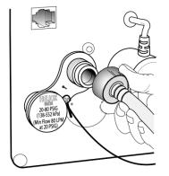
If you have the upgrade for Heliox delivery, attach the Heliox hose .to the tethered "Smart" connector fitting on the left of the back panel as shown in Figure 2–30.
