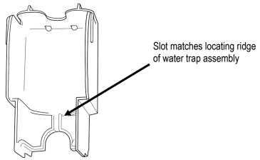
Figure 2–4: Exhalation Filter Cartridge Showing Locating Slot
