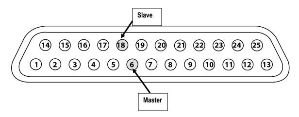
Figure 2–33: ILV Connection Pin Configuration
