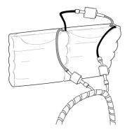
The Avea has an internal, Nickel Metal Hydride battery pack that will provide power backup for short periods in the event that the mains power supply is lost (Figure 8–1). Under normal operating conditions and when fully charged, the internal battery is capable of powering the ventilator alone for 1 hour or the ventilator and compressor for 30 minutes.
