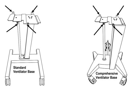
Figure 2–1: Basic and Comprehensive base attachment
