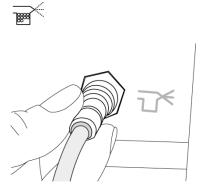
Figure 2–22: Attaching nebulizer tubing
