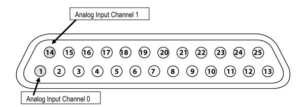
Figure 2–36: Analog Input connections
