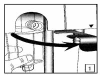
Figure 2–10: Inserting the Filter / Water Trap combination
